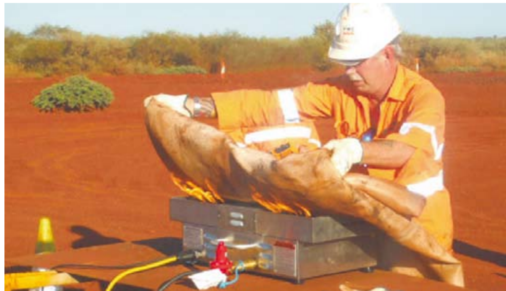
Bruce McBeath from Mesa A using a fire blanket on the BullEx Fire System.
